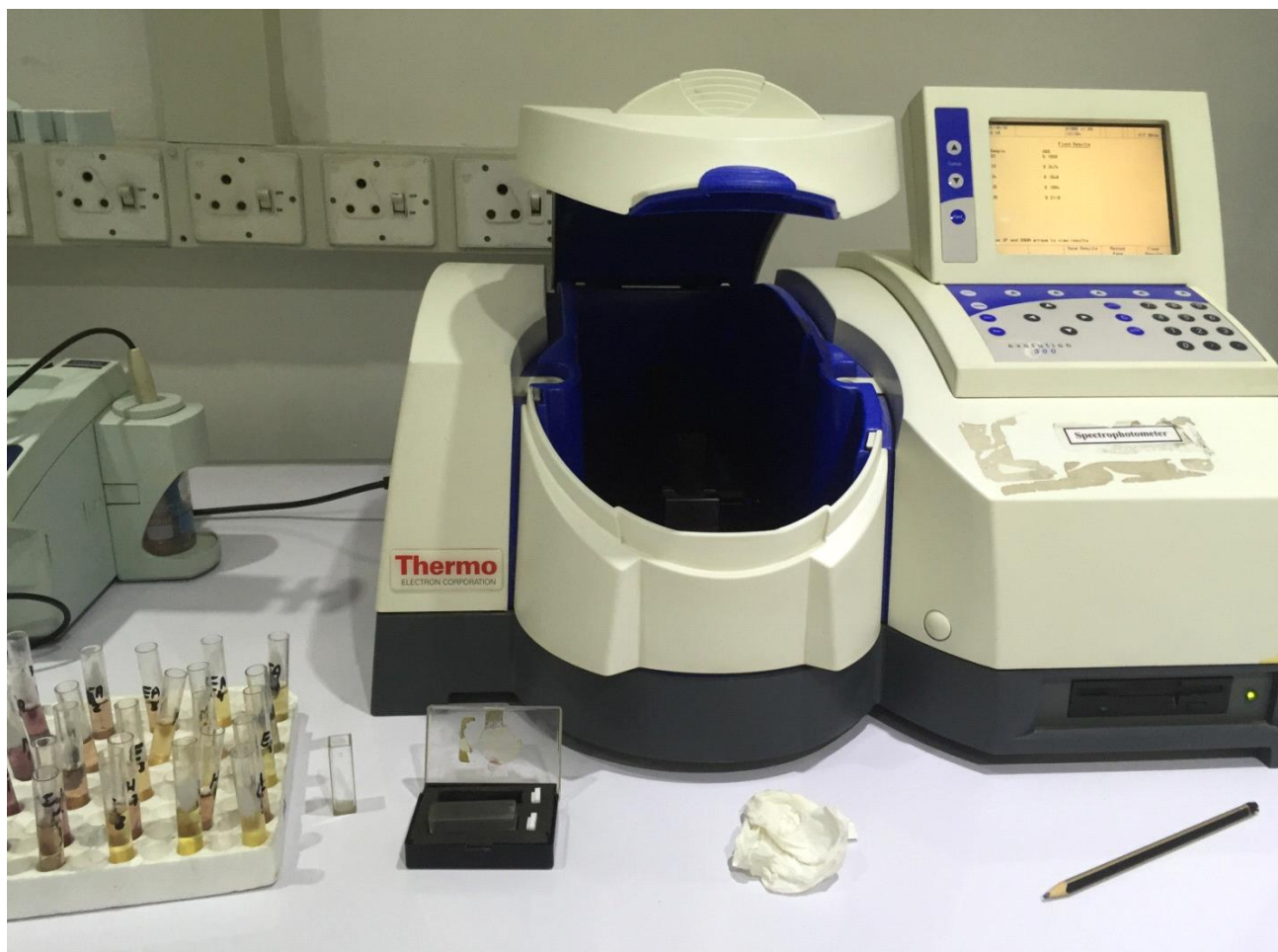
Figure 3.3-1 Spectrophotometer (Thermo-Nicolet Evolution 300) Samples are ready to get their spectrum with the help of Spectrophotometer.
